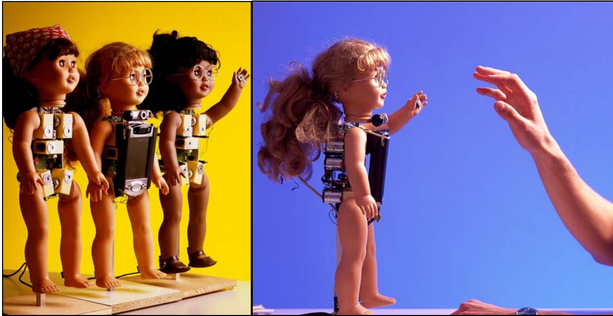
Figure 2: LEFT: 3 Robota robots. The middle one is provided with a Compaq iPAQ 3850 as main CPU. RIGHT: A camera mounted on the PocketPC of Robota enables tracking of the hands and nose of the user through optical flow and recognition of skin colour. Robota can, then, mirror the movements of the arm and head of the user.
