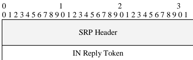
Figure 4. Extended SRP Header: the INRT allows intermediate group member nodes to validate the request and provide a reply.
