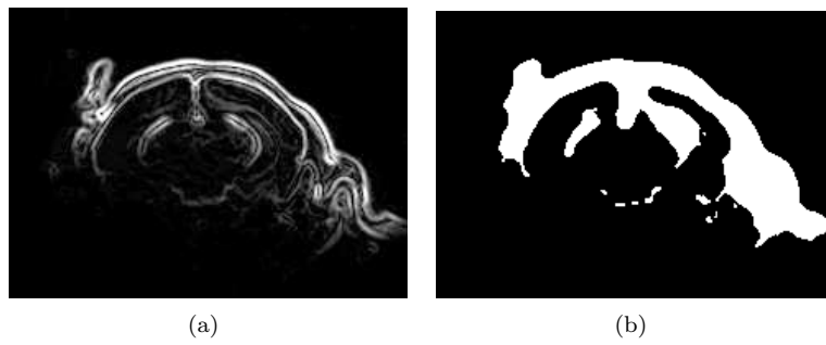
Figure 3.5: Gradient of the image (a) and Gradient image thresholded and filled (b).
