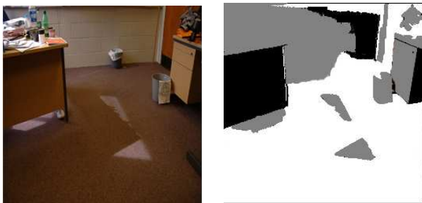
Figure 7. The left image is an indoor scene and the image on the right shows the illuminant map recovered: outdoor (gray), indoor (black) and mixed (white).
