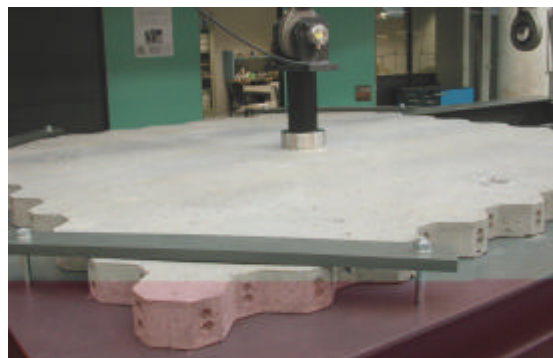
Figure 13. Punching test on BHP slabs, 70 mm thickness.
