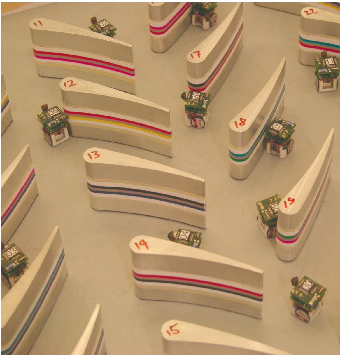
Figure 3.4: The experimental setup endowed with colored markers that allow for unique identification of a blade using the on-board camera.
