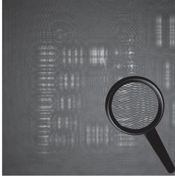
Figure 2.4: Typical 1024x1024 off-axis hologram of a USAF test target acquired in reflection configuration. Inset: a zoom showing clearly the interference fringes
