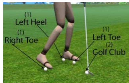
Figure 3. A typical constraint configuration used to edit a golf swing. 1 means the highest priority and 2 is the second one, see Algorithm 1 for more details.
