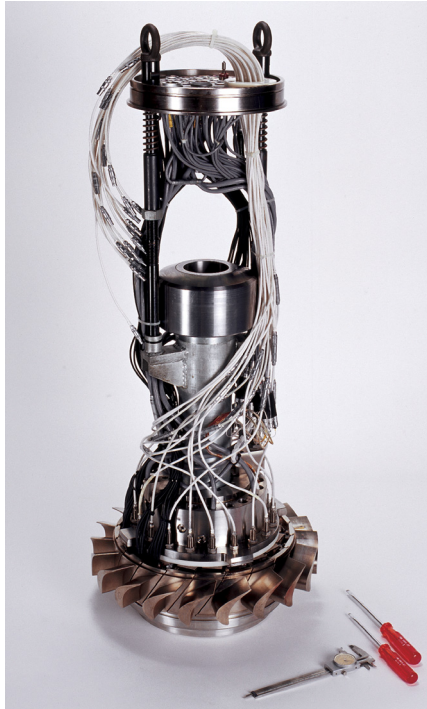
FIGURE 14. B-E ADTurB tower
