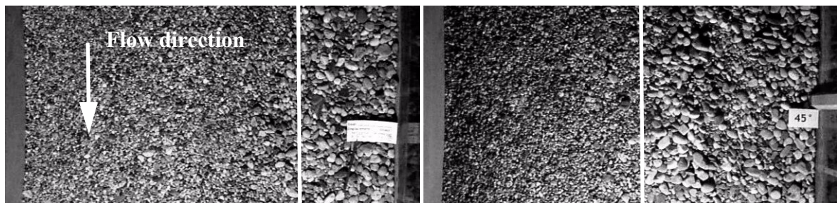
Figure 6.21: Bed surface in the first scour hole (tests B1d and B2d) without (left) and with ribs (right)
