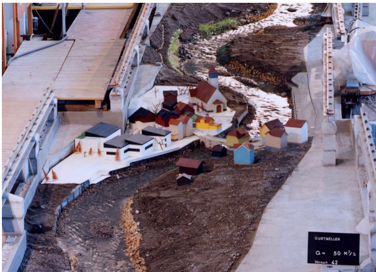
Figure 1.1: Hydraulic scale model of the Reuss River, Gurtzellen, Switzerland [Kuster et al., 1992]
