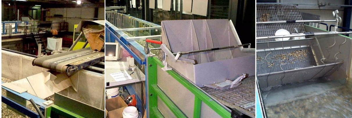
Figure 4.2: Sediment inlet (left) and sediment sampling at the outlet (center and right)
