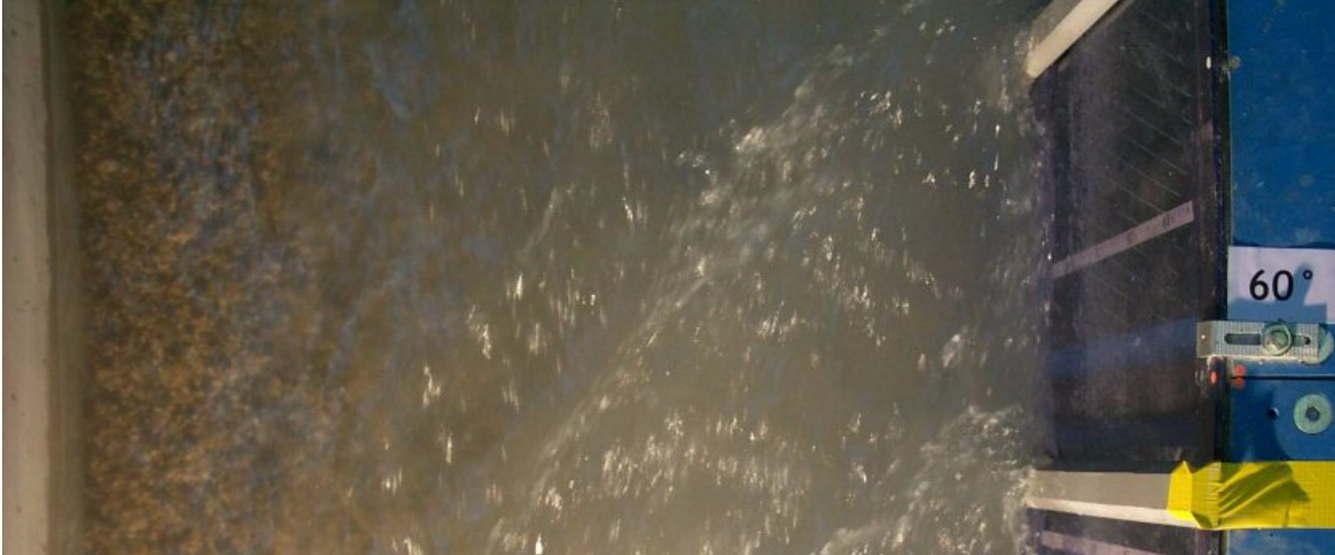
Figure 6.14: Vertical view on the water surface waves; ribs-spacing 4°, test C2c
