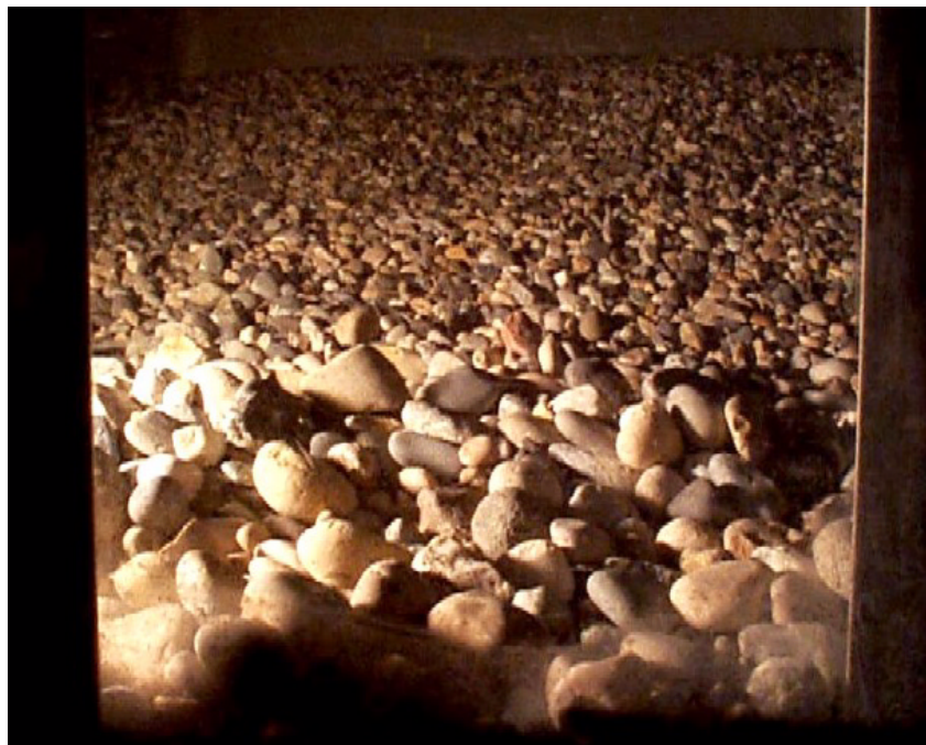
Figure 5.2: Grain sorting, view across the outer side wall at 45° (test with macro-roughness - A2)
