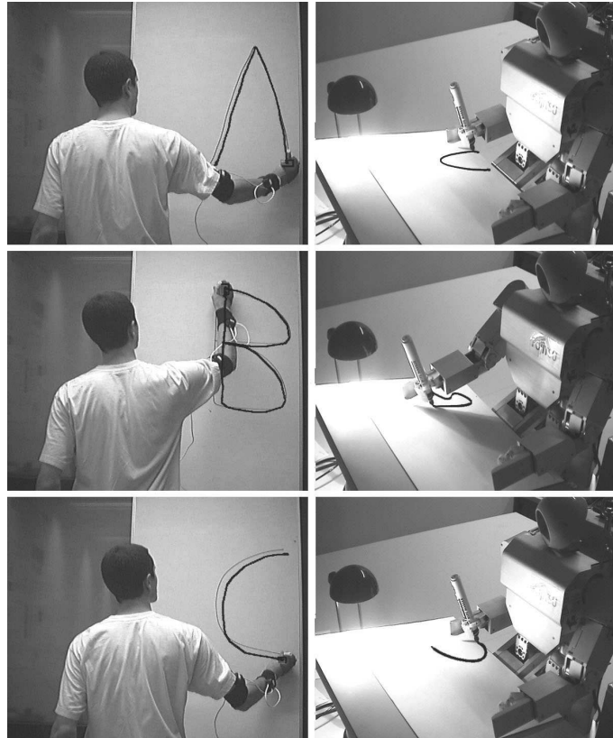
Fig. 2. Demonstration ( left column ) and reproduction ( right column ) of drawing the three stylized alphabet letters A, B and C. The motion reproduced by the robot follows a trajectory generalized across the different demonstrations. As the trajectory is projected by PCA in 2 dimensions, the letters can be written on a different plane.
