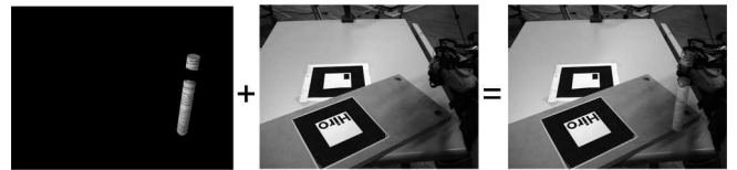
Fig. 5 Photo taken from the user point of view, and augmented with what is displayed in the HMD
