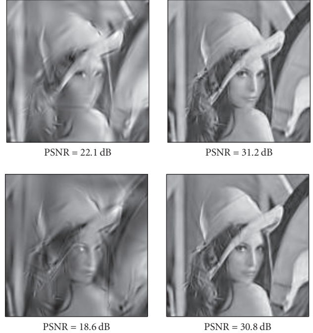
FIGURE 8: Reconstructed Lena images, as a function of a number of received descriptions, from 1 description on the left column, to 2 descriptions on the right column. (Top row: our scheme, Bottom row: atom sharing scheme.)
