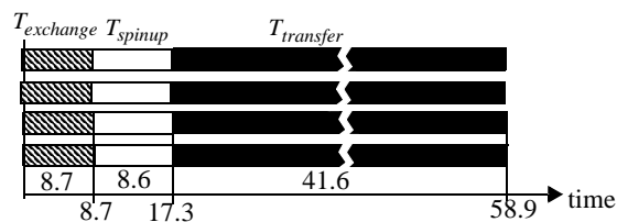
Fig. 5. Time for retrieving a 500 MB file striped across 4 disks located in different NSM Satellite jukeboxes.
