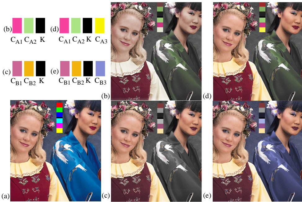
Figure 13. Original image (a) mapped into 4 different target color gamuts: two custom inks and black (b),(c); three custom inks and black (d),(e).
