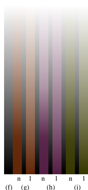
Figure 14. Gray axis (f) mapped into 3 different target gamuts according to (n) non-linear and (l) linear lightness rescaling.
