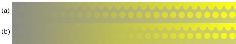
Figure 15. Original hue line (within the disks) obtained by (a) a linear saturation mapping, (b) a non-linear saturation mapping.
