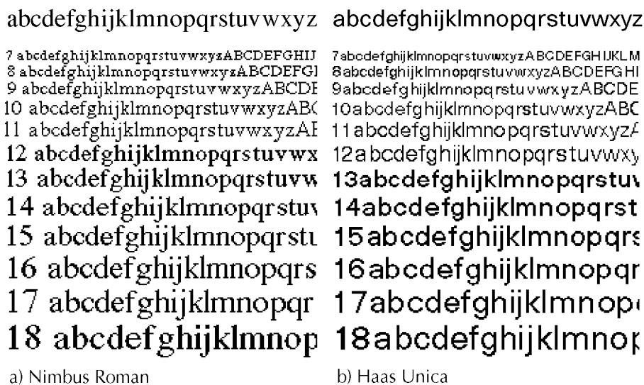
Figure 33. Nimbus Roman and Haas Unica rendered at low resolution (size: caps-height in pixels)
