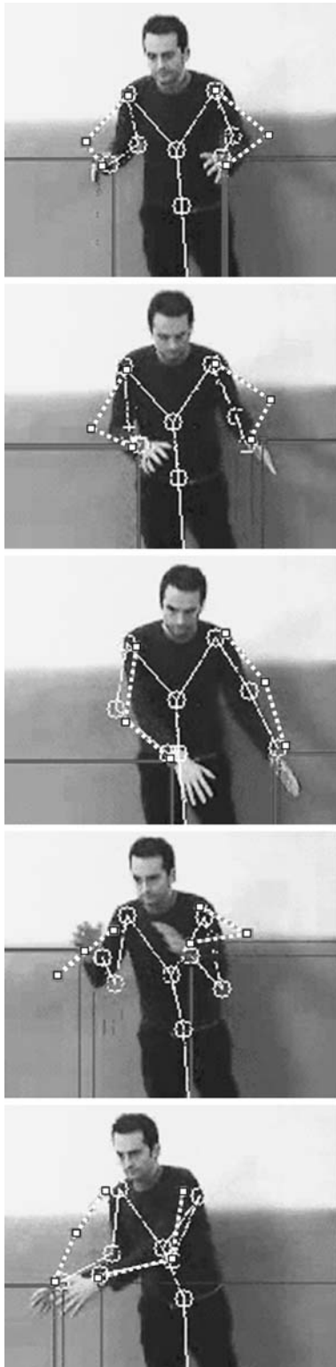
Fig. 13 Moving an imaginary box (real-time duration, 5.5 s). Squares —analytic solution, circles —numeric solution
