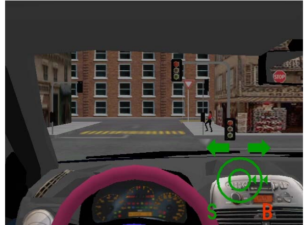
Figure 12 a): The car "sees" the traffic lights and the pedestrian inside a circular zone. The panel informs the driver that he/she must brake (B – in red at bottom right corner).
