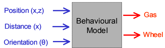
Figure 10: Behavioural model for the car driving simulation inside a virtual city with inputs and outputs. The MDP has two different actions: gas and wheel.
