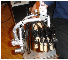
Figure 8: Problem of an external rotating force due to the hardware
