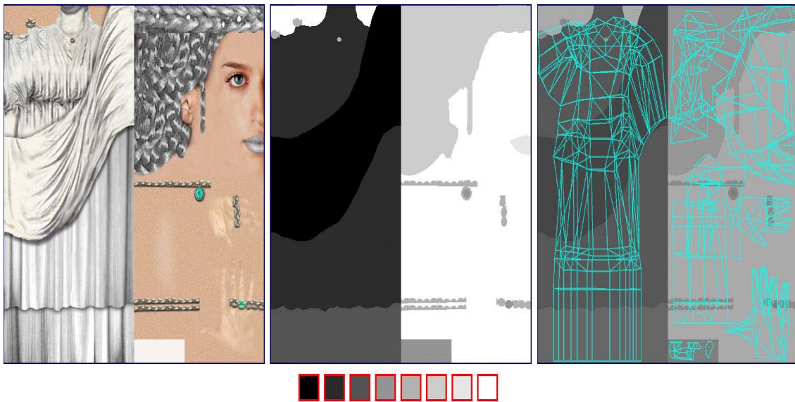
Figure 4: The base variety texture displayed along with the alpha map in the middle and the triangles laid out on the right. The 8 small squares beneath the alpha map show the alpha colors.
