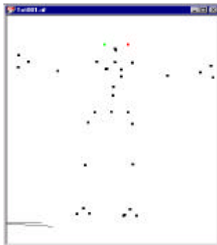
Fig. 2. A frame containing 3D optical markers from a gym sequence, used as input for the skeleton fitting
