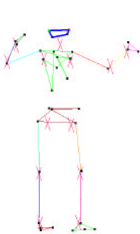
Fig. 15. Crosses show the position of some joints estimated using the local fitting technique
