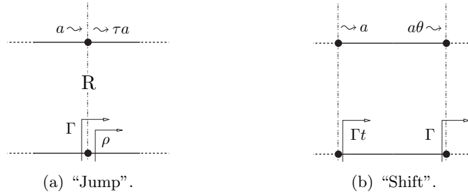
Figure A.2: Wave and reflection coefficient propagation (a) through an interface between adjacent TLs and (b) along a TL.
