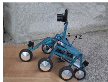
Figure 5. The Shrimp mobile robot
