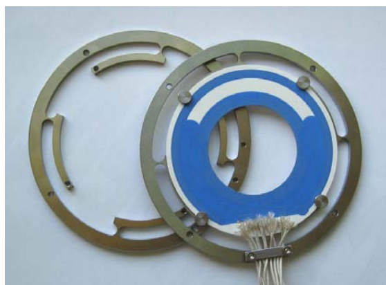
Fig 7. Sensor holder for thermal expansion compensation, with and without position sensor.
