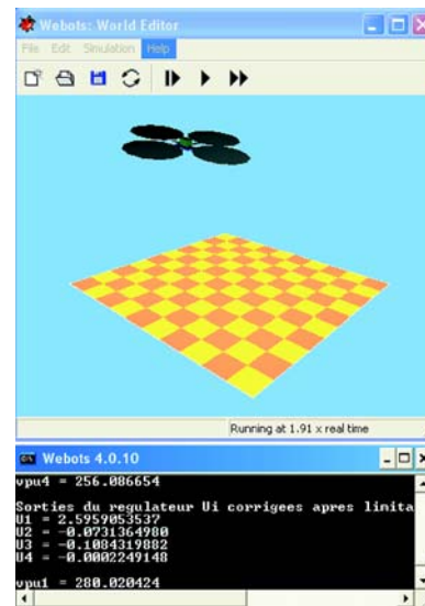
Figure 14. 3D simulation of a Quadrotor on webots already permits the test of the controller under disturbances
