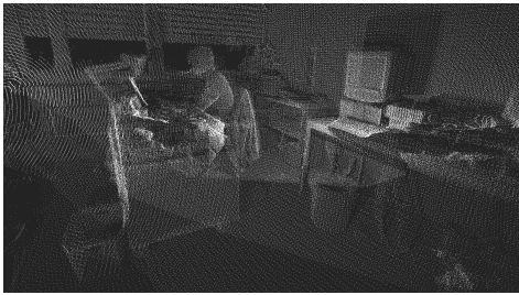
(c) Part of an office reconstructed by several registered 3d scans showing high detail.
