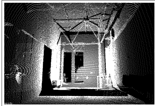
(b) The same scene visualized as a point cloud measured by the rotating laser scanner.
