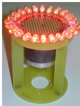
Figure 4: The circular set of LEDs forming the light source, positioned on the mirror.
