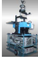
Figure 7: The fully autonomous robot Donald Duck. The panoramic vision system has been mounted right above the wheels. So, for a given position, the fingerprint extraction does not depend on the robot's orientation.
