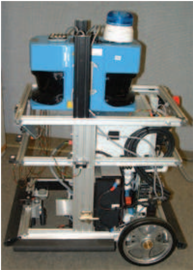
Fig. 7. The robot BIBA equipped with the laser range finders
