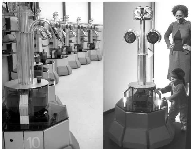
Fig. 1. On the left side: the RoboX team at the charging station during the Expo.02 event. On the right side: one RoboX interacting with visitors and taking a photo of them.
