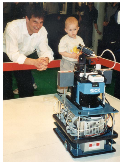
Figure 4: Daffy, after detecting a young visitor, interacts with him by speaking, tracking him and moving the pan-tilt head for mimicking expressions. It detects human movement by means of the CCD camera and closes the interaction loop with its speech synthesizer and gestures as a combination of robot and pan-tilt movement.
