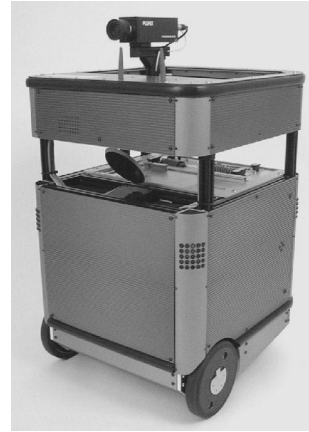
Fig. 4. Pygmalion, the robot which was used in the experiments. It is a VME based system carrying currently a PowerPC card at 300 MHz with 32 MB of RAM. Besides wheel encoders and bumpers, the sensory system includes a 360° laser range finder and a gray-level CCD camera discussed in Section 2. During all experiments it ran in a fully autonomous mode.
