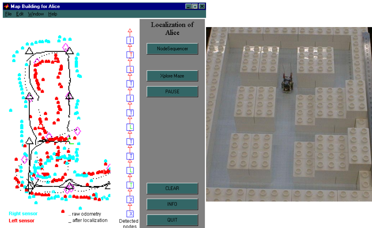
Figure 5. Global localization in the a priori known environment visible in the picture nearby and depicted in Figure 6. Corrected recognizable locations are marked by a triangle. The robot started from an unknown position. The vertical chain shows the sequence of the last thirteen detected places.
