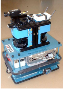
Figure 4: The autonomous robot Donald Duck. Its controller consists of a VME standard backplane with a Motorola PowerPC 604 microprocessor clocked at 300 Mhz. Among its peripheral devices, the most important are the wheel encoders, a 360° laser range finder and a grey-level CCD camera (not used here).
