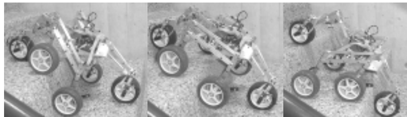
Figure 10 : Climbing sequence in stairs (h=17 cm, w=21 cm)
