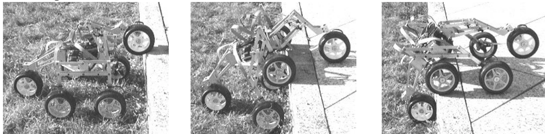
Figure 9 : Climbing sequence for a step of 22 cm high (2 times the wheel diameter)
