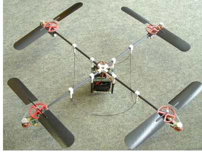
Figure 3.9: Initial design of OS4.
