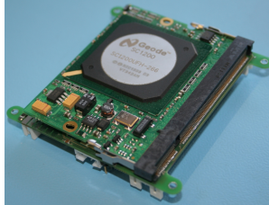
Figure 3.13: The x-board based, 40 g and 56x71 mm computer module.
