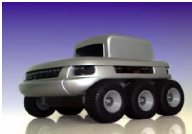
Figure 5. The new Koala robot has a structure very similar and compatible to Khepera but a much bigger scale.
