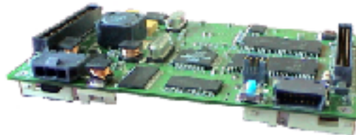
Fig. 10 - The KoreBot card from K-Team, a full-UNIX computer with internet and wireless abilities weighing 40 g.
