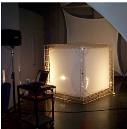
Fig. 5 – Photograph of a Mascarillon M170 ready for take-off, May 2005. The white bladder is filled with helium, and is stretched within the ultra-light basswood structure.
