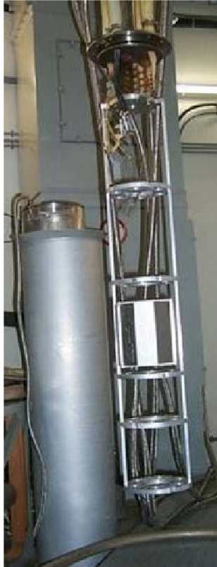
Figure 5.2: Photograph of the sample canister showing the inside structure with multiple shelves for sample storage. The canister is sealed against water ingress and maintained at constant temperature during the experiment, with dry nitrogen atmosphere at constant pressure.
