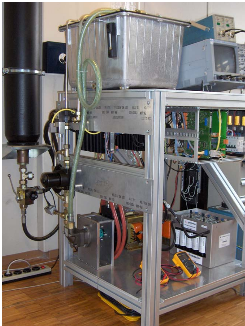
Figure 6.5.: Picture of the test-setup for hybrid BOP-A and Supercapacitors
