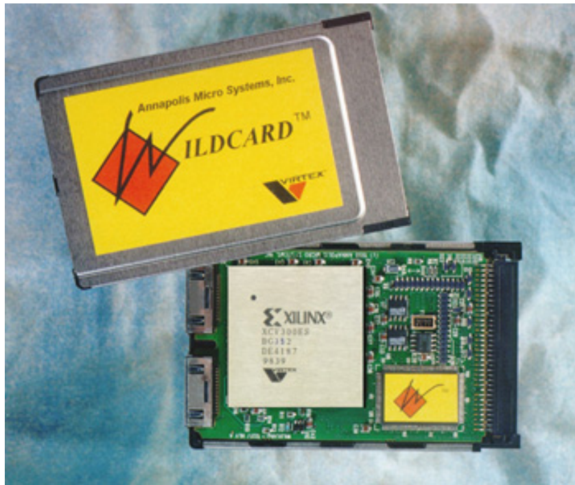
Figure F.1: Wildcard II reconfigurable PC Card from Annapolis Micro Systems. The card contains a Xilinx Virtex-II device, PC interfacing logic, and on-card memories.
