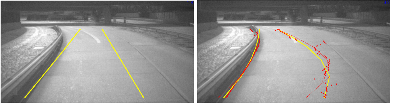
Fig. 2. Lane detection without (left image) and with (right image) cumulated gradient along the lane. Using this global hypothesis, the algorithm succeeds in situations where the contrast of one street side (left one) is not constant and the other side (right one) has no particular marking.
