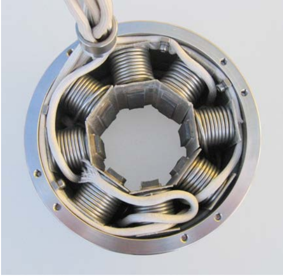
Figure 7.6: Radial bearing with Thermocoax wire.
