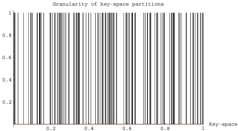
Fig. 4.4. Key-space partitioning granularity of a randomly generated unbalanced P-Grid network with 120 partitions. Each vertical line in the figure corresponds to a partition of the key-space in the instantiated P-Grid.
