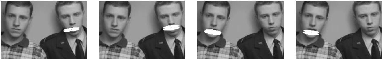
Fig. 7. Results for Experiment 2 : four frames taken from a clip with two speakers in front of the camera taking turn in reading digit string. In the first two frames the right person is speaking, while in the last two the left one is speaking. The footprint of the most correlated atom is highlighted in white. The mouth of the correct speaker is detected.
