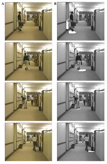
Fig. 4. Shadow segmentation results for the test sequence *Hall Monitor*. (A) Original image; (B) shadow mask (white pixels) superimposed on the original image.
