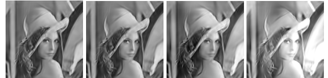
Fig. 5. Example of reconstructed images when adding randomly values to the projection parameter.
