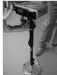
Fig. 1. Laser range scanner mounted on vibration damping monopod in OR.
