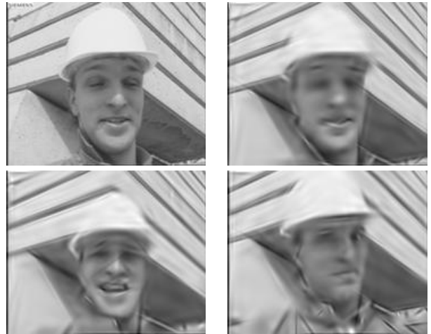
Fig. 4. Prediction results: Original 0 frame (upper left), Coded 0 frame (upper right), Predicted 20th frame (down left) and Predicted 98th (down right).
