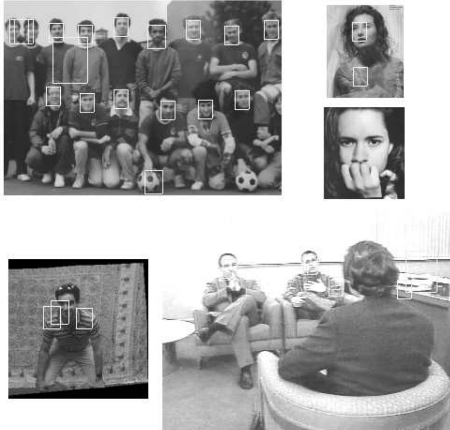
Figure 4.10: Results of the detector using a cascade of 14 classifiers. Example of poor detections. Some faces are missed and false alarms are detected.
