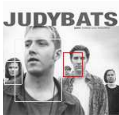
Figure 4.5: Example of bad multiple detection integration. The black bounding box contains two faces.
