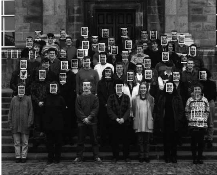
Figure 4.9: Results of the detector using a cascade of 14 classifiers. Example of good detections with some false alarms.
